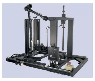
To protect evidence items under examination against contamination with traces of foreign DNA, the object area is covered with plain black aluminium profiles. In addition, an easy-to-clean plastic cover is available to protect the turntable surface and a silicone cover for the iaw chuck.
