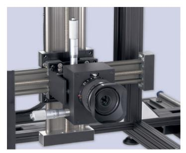
The ForensiScan is equipped with a high resolution RGB camera and a motorised lens.
